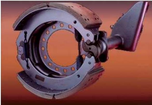
Figura 35 - Pneumatic S-Cam Brake
