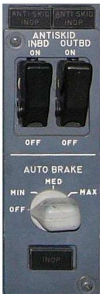
Sistema "A" Inboard Brakes e Sistema "B" Outboard Brakes
